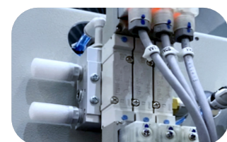
4 Into 4 Out Pneumatic Valve Group and M Code
